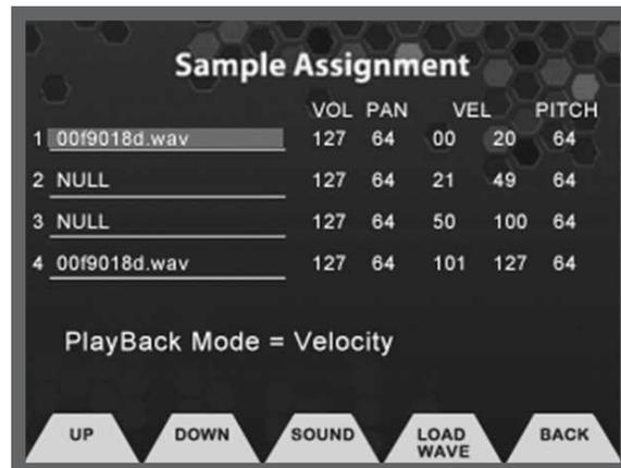
Playback Mode allows you select between Velocity switching, Sequence and Random between the samples that are assigned in the User Wave Instrument.
